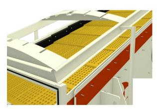
Picture 1. Example of the top canopy construction with arches
